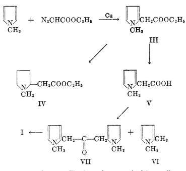
chloride-pentane as the crystallization solvent resulted in excellent recoveries of pure acid (V) which was then converted to the barium salt and pyrolyzed under reduced pressure. The pyrolysate was easily separated into crystalline ketone (VII) (12% yield) and 1,2-dimethylpyrrole (49% yield). Späth and Tuppy (7) report a higher yield of crude ketone by pyrolysis of the lead salt on a much smaller (one one-hundredth) scale.
